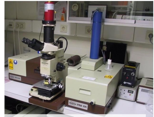
FTIR-Raman spectrometer Bruker IFS 66 and Raman module FRA106
