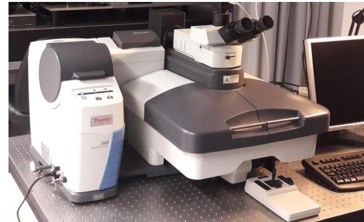
Dispersive confocal Raman microscope Thermo DXR
